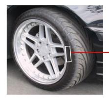
All tires have the maximum load shown near the bead on both sides.
