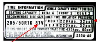
The car manufacturer's pressure requirement is calculated to allow sufficient load capacity, and to achieve desirable vehicle handling qualities.
